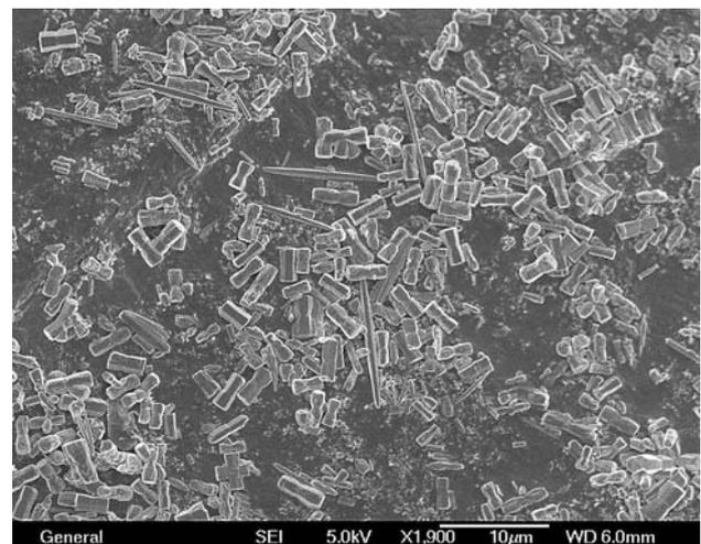
**Fig. 2** Scanning electron microscopy (SEM) image of ZnO microrods
