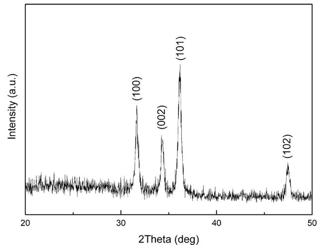
**Fig. 1** X-ray powder diffraction (XRD) pattern of surface etched ZnO microrods
