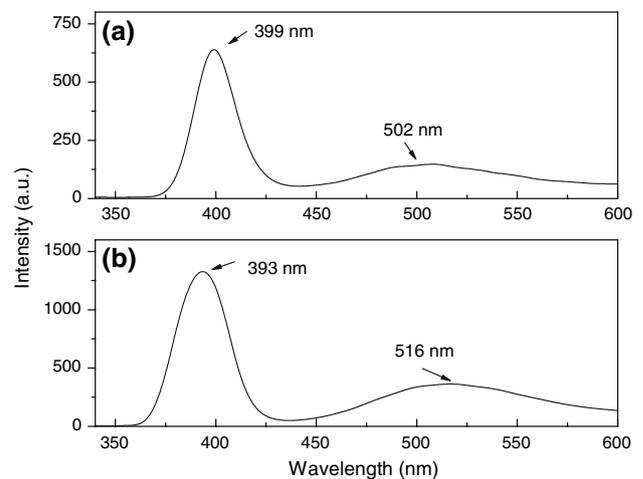
**Fig. 5** Photoluminescence (PL) spectra of (a) ZnO microrods and (b) surface etched ZnO microrods
